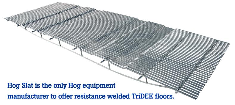
Introducing a galvanized triangular bar (TriDEK) flooring system that is used in nursery and farrowing applications. TriDEK floors are made from rolled steel rod which has a tensile strength of 80,000 psi and hardness of 95 Rb. The rolled TriDEK rods are then resistance welded to a 13/32" diameter cross rod.
