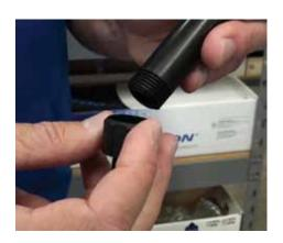
**Step 8:** Insert the bottom seal, raised portion facing up, into the black cap and thread onto the stem, hand tight.
