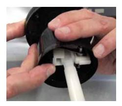
**Step 27:** Test the piston by pressing on the top and bottom of the push rod. It should click both times.
