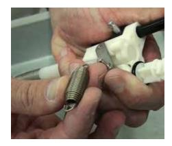
**Step 13:** Unhook and remove the actuator springs (Part #: M009).
