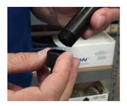
**Step 6:** Unscrew the black cap and remove the bottom seal (Part #: J003) between the black stem and the cap.
