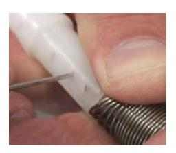
**Step 17:** Now push the metal pin (Part #: M005) out using the paper clip. This allows you to remove the spring from the slide valve.
