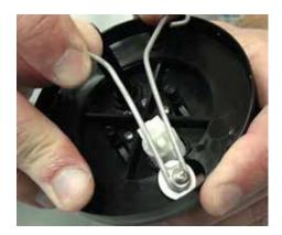
**Step 10:** Spread the wishbone and remove from the inlet valve.
