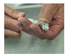
**Step 16:** To remove the slide valve from the plunger rod you will need a large paper clip or awl. Push the spring down and hold firmly.
