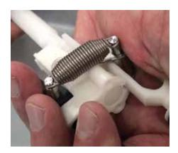
Step 22: Install the actuator springs.
