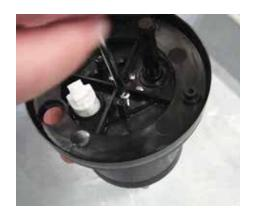
**Step 25:** Now reinstall the four screws and tighten in a star pattern.
