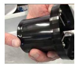
**Step 5:** In order to check the piston shell, remove the piston and check the upper and lower flanges on the piston shell. If they are worn or have scratches the piston shell needs to be replaced.
