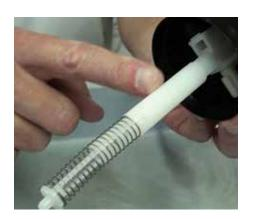
**Step 8:** Next, pick up the piston and inspect the plunger rod (Part #: P009) and slide valve (Part #: P010). The plunger rides inside the top seal to create suction. If there is a build up of scale or has deep scratches, it may not draw the correct amount of solution. If your plunger rod does have scale build up, just soak the piston assembly in a solution of Medicator Rx (Part #: CLEANSER-LS) for 24 to 48 hours. If the plunger rod has scratches it will need to be replaced.
