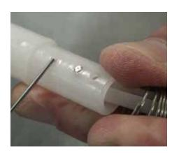
**Step 5:** Push the slide valve into the plunger rod and reinstall the pin. The center hole is the 1:128 setting. If you need 1:200, install the pin into the top hole, if you need 1:100, install the pin into the bottom hole. Make sure the pin is flush so the spring doesn't get stuck.
