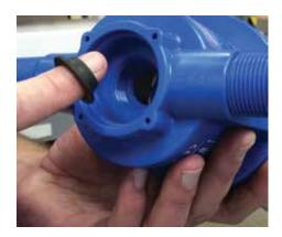
**Step 4:** Remove the top seal (Part #: J002) that is located between the blue body and the black stem.
