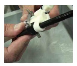
**Step 14:** Remove the push rod (Part #: P008) by sliding it out.
