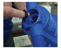
**Step 6:** To reassemble, place the top seal with the raised center portion facing upward inside the body.
