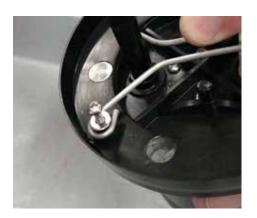
**Step 26:** Reinstall the wishbone spring, then reinstall the washers and screws, hand tight.
