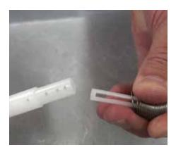
**Step 18:** To reinstall the slide valve onto the new plunger rod slide the spring over the slide valve. Push to the bottom and grasp firmly.
