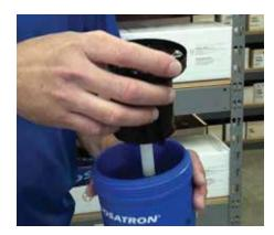
**Step 7:** Insert the piston back into the blue body.
