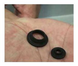
**Step 7:** Inspect both seals for nicks, grooves, and wear. Make sure they aren't gummy, sticky, or missing. If the seals are dirty, you may be able to just clean them and reinstall. But if they are damaged or missing, it is definitely time to replace.
