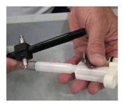
**Step 21:** Install the push rod with the long portion up making sure to insert it with the groove side inward.
