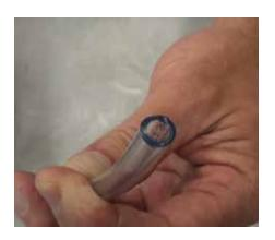
**Step 12:** One last thing. Take a look at the top of the suction tube. If it flares out, cut off an inch or so and reinstall. Or, if the suction tube is cracked, has holes, is rigid, or looks really old, replace.
