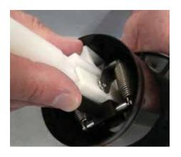
**Step 23:** Align the push rod and inlet valve inside the piston shell and slide the actuator assembly in completely.
