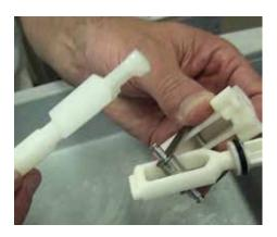
**Step 15:** Remove the plunger rod (Part #: P009) by lifting it up slightly and out. Set aside the actuator (Part #: MP001).
