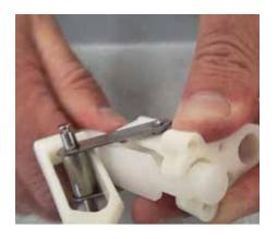
**Step 20:** Pick up the actuator and install the new plunger rod by sliding it into the actuator and pulling it down to lock. Make sure the head of the plunger rod is flush.
