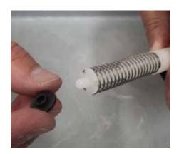
**Step 1:** Inspect the bottom seal (Part #: J003), slide valve (Part #: P010), and spring (Part #: M003).
