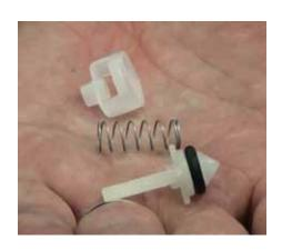
**Step 9:** Once you have the parts out, make sure they are not damaged, gummy, sticky, or missing. If the parts are dirty, you can clean and re-install. But if they are damaged or missing it's time to replace. Remember to keep these parts clean and in good shape so your check valve will do its job.
