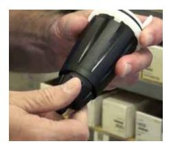
**Step 6:** Now unscrew and remove the check valve nut.
