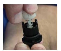
**Step 12:** Replace the retainer (PDI739) by aligning it and turning it a ¼ turn clockwise to lock.
