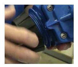
Step 19: Hand tighten the stem nut.
