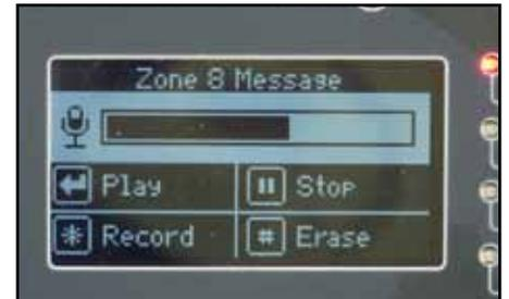
Select the \* Record button and record a message that will play when an alarm condition is signaled. In our example we used "Feed Outage, Jones Site, Building 1, Bin 1"
