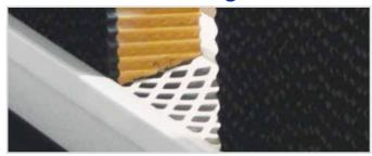
Large square poly trough offers greater capacity than round troughs and allows for trough to set directly on concrete foundation without brackets. Diamond Cut trough cover increases drainage area by 33% to eliminate water pooling at the bottom of the pad. Water recycles quicker and pad life is extended because the pad bottom does not remain soggy.
