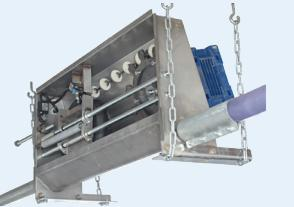
Constructed of 304 stainless steel with a high efficiency 1-1/2 HP motor. Steel sprocket wheels with two safety switches, one each on the chain tensioner and access cover. Features a clamping rod for safety instead of cable or spring system. Connects seamless with the steel fill hopper.
