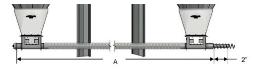
After insertion of the anchor bearing, insert the auger lock and tighten until auger is secure. Do not over tighten as auger will deform and be unable to rotate freely.
