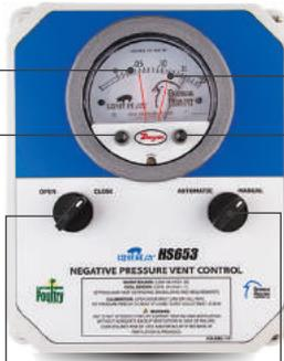
Pressure reading exceeds this limit, the vent machine OPENS vents to lower the pressure inside.
