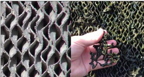
Scale is the buildup of minerals hard water leaves behind as it evaporates during the cooling process. Heavy deposits of scale require the use of a broom to dislodge the debris and then rinsing them off the pad with a low-pressure hose nozzle. The best way to deal with scale is to prevent it from forming in the first place. Adding a descaler treatment to the water helps keep the minerals in suspension and prevents them from sticking to the pad.
