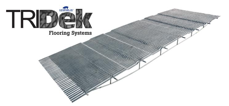
Introducing a galvanized triangular bar (TriDEK) flooring system that is used in nursery and farrowing applications. TriDEK floors are made from rolled steel rod which has a tensile strength of 80,000 psi and hardness of 95 Rb. The rolled TriDEK rods are then resistance welded to a 13/32" diameter cross rod.
