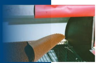
The egg collection system used on our two-tier nest is simple, effective and unique. Curved mini conveyors bring the eggs to one level providing a seamless and smooth transfer. A variety of customised collection systems are available for both our own and other nest makes.
