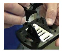
**Step 7:** To remove the rocker, spread the supports and pull it up.
