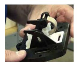
**Step 4:** Remove and replace the slider assembly (PPDI048) that includes the white plastic slider, rocker, and the blade spring.
