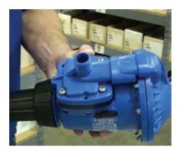
**Step 17:** Now, reinstall and tighten the six screws in a star pattern.
