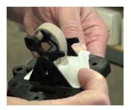
**Step 12:** Test the new assembly by pushing the slider back and forth. It should click each time and not bind.
