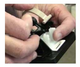
**Step 10:** Hook the blade spring on the rocker and press the axle into the top of the slider.
