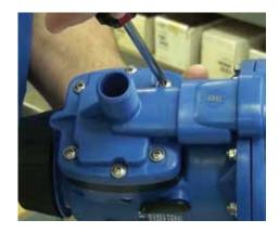
**Step 1:** If the unit isn't clicking, unscrew and remove the 6 screws from the outlet plate assembly.
