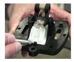
**Step 13:** Next, position the slider so that the small tooth touches the stop.
