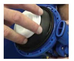
**Step 3:** To remove, unscrew the diaphragm assembly and discard. Install the new part and hand tighten.
