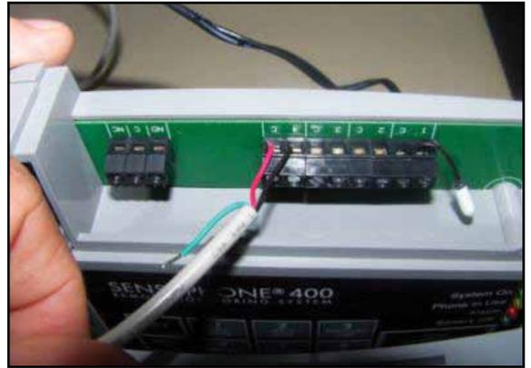
For our example we have selected Zone 4 to be the bin alarm. Install the red lead into C terminal and install the black lead into the 4 terminal. The wire used between the magnetic sensor and the Sensaphone should be a 26 ga wire which is common telephone wire.
