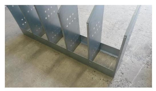
2. Next, insert the nest bottoms (item 3) as shown. The angled edges should be on the left and right side of each space.
