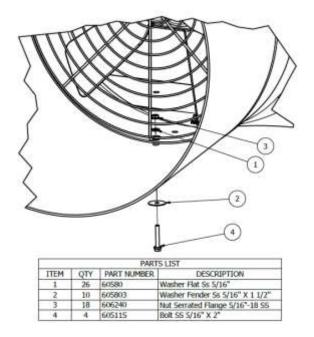
6. Insert fan shroud into rough opening from inside of house. This can be done with cone already installed as the major diameter of the cone is smaller than the required rough opening.
