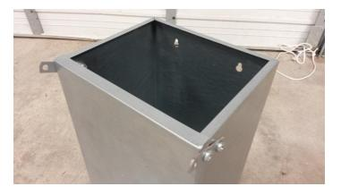
7. Make sure all nuts and bolts are tightened with the 1/2'' socket and wrench.
