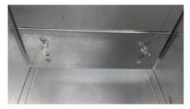
Fasten FS400-9 to front of feeder. The brackets installed in step 3 should be on the outside of the front panel. Now tighten both bolts securing the FS400-2 brackets. Install FS400-1 with nut and bolt as shown. Also place these brackets on the outside of the front panel. Tighten with 1/2" socket and wrench.
