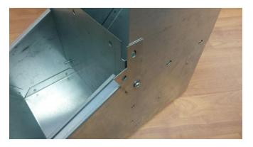
4. Using the 1/2" socket and wrench, tighten nuts and bolts around bottom as shown.
