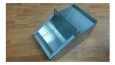
2. Place FS400-8 around the outside of FS400-7aligning the holes.
