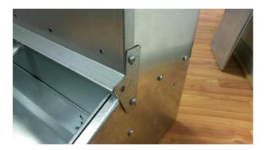
8. Similar to Step 7, secure bracket FS401-1with a nut and bolt as shown.
