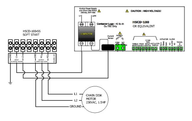
ALL WIRES SHOULD BE 12 AWG STRANDED, 300V
