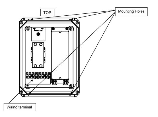
When installing external wiring, <u>use liquid tight connectors only.</u> Drill holes for connectors in this location to have adequate space for wires. Take special care when drilling holes into the enclosure to prevent damage to internal components.
