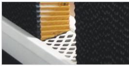
Large square poly trough offers greater drainage capacity and allows trough to sit directly on concrete foundation with or without brackets. Diamond cut poly trough cover increases drainage area by 33% allowing water to recycle quicker extending pad life.
