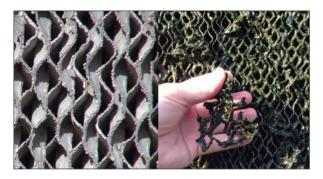
Scale is the buildup of minerals hard water leaves behind as it evaporates during the cooling process. Heavy deposits of scale require the use of a broom to dislodge the debris and then rinsing them off the pad with a low-pressure hose nozzle. The best way to deal with scale is to prevent it from forming in the first place. Adding a descaler treatment to the water helps keep the minerals in suspension and prevents them from sticking to the pad.
