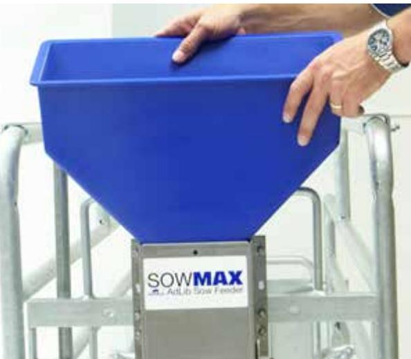
The SowMAX dispenser holds approximately 6.5 pounds of feed. Adding the blue plastic hopper, feed capacity increases to 20.5 pounds. Topping off the hopper with feed both morning and evening, will provide any sow with a full day's ration.
